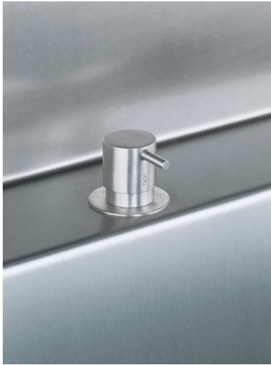
S50 Stop valve with ¼ turn ceramic disc technology. Includes non-return valve and ½" inlet/outlet. 60 mm circular flange 001G. Hole cut out size: 30 mm.
